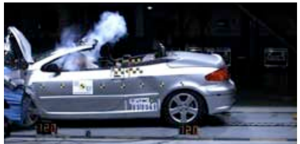
Offset crash test at 64km/h
