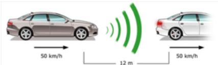
Approaching a braking vehicle with long headway: 1.51 out of 2 for AEB, 1.92 out of 2 for FCW
