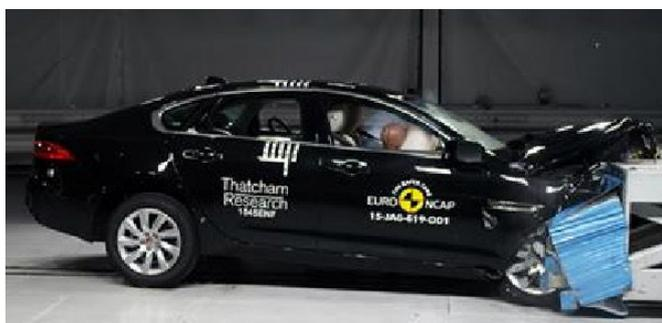
Frontal offset test at 64km/h (Copyright Euro NCAP)
