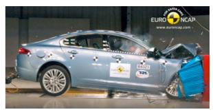
Offset crash test at 64km/h
