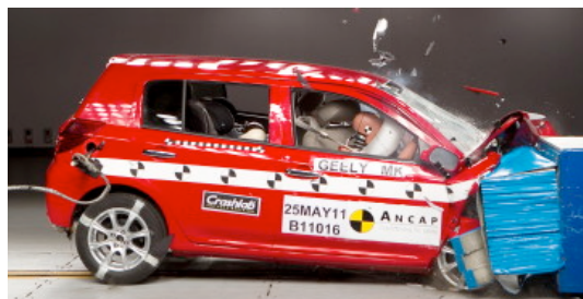
Offset crash test at 64km/h
