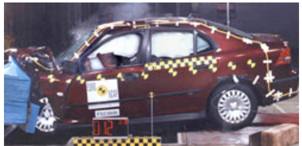
Offset crash test at 64km/h
