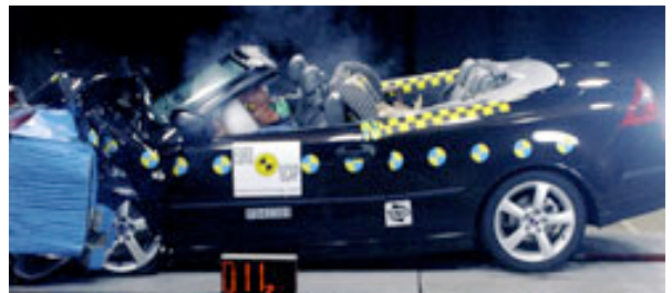
Offset crash test at 64km/h
