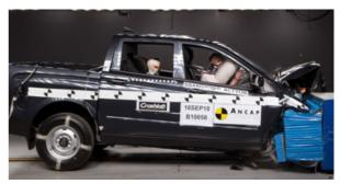
Offset crash test at 64km/h
