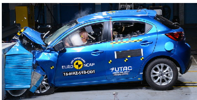
Frontal offset test at 64km/h (Euro NCAP)
