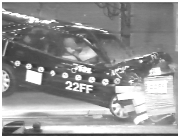
Offset crash test at 64km/h
