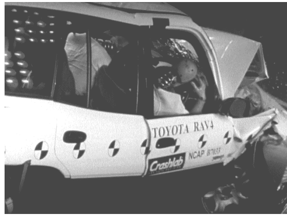
Offset crash test at 64km/h
