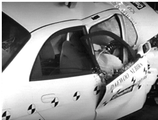
Offset crash test at 64km/h
