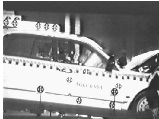
Full-frontal crash test at 56km/h
