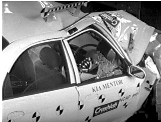
Offset crash test at 64km/h
