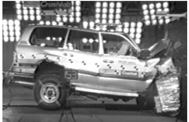
Offset crash test at 64km/h
