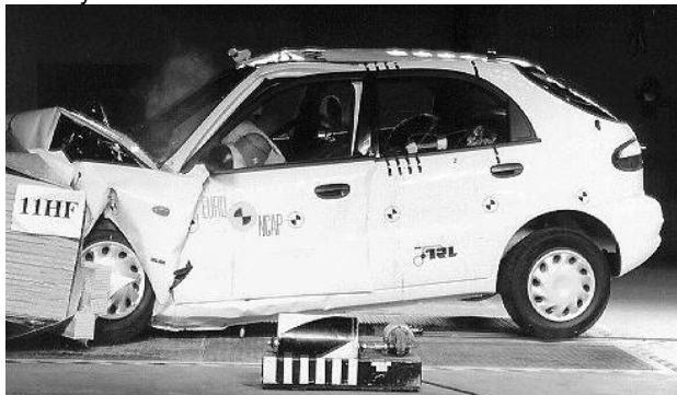
Offset crash test at 64km/h
