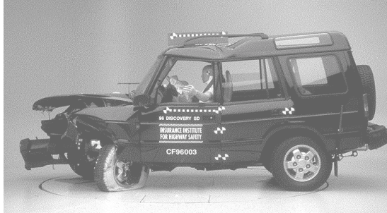
Offset crash test at 64km/h
