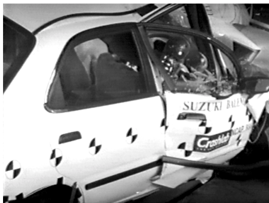
Offset crash test at 64km/h
