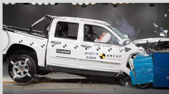
Frontal offset test at 64km/h
