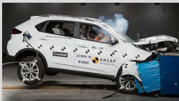
Frontal offset test at 64km/h
