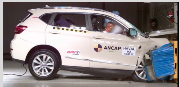
Frontal offset test at 64km/h
