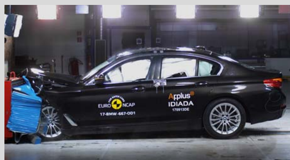
Frontal offset test at 64km/h
