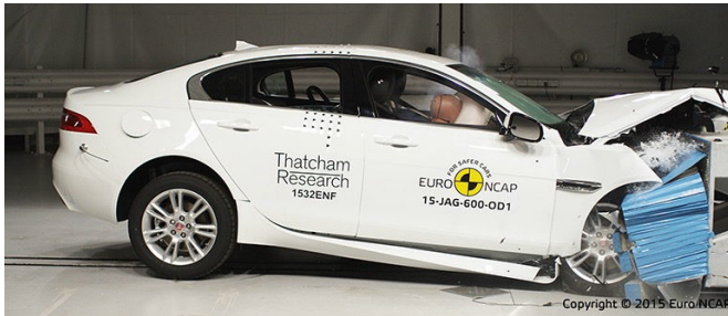
Frontal offset test at 64km/h (copyright Euro NCAP)
