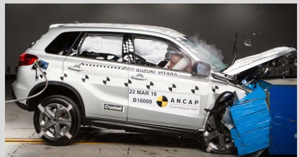
Frontal offset test at 64km/h
