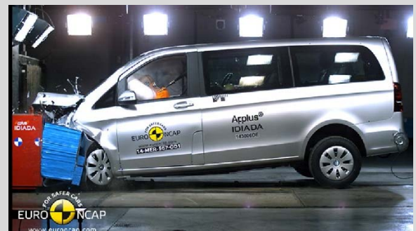
Frontal offset test at 56km/h (Mercedes-Benz V-Class)
