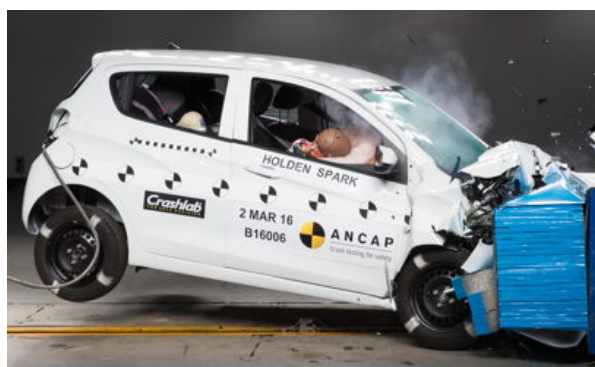
Frontal offset test at 64km/h
