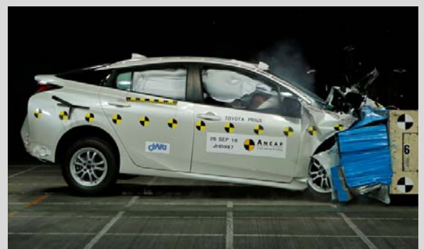
Frontal offset test at 64km/h
