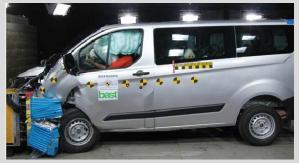
Frontal offset test at 56km/h
