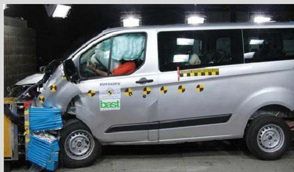
Frontal offset test at 56km/h (Ford Transit Custom)
