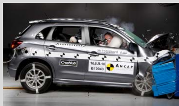
Frontal offset test at 64km/h
