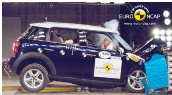
Offset crash test at 64km/h
