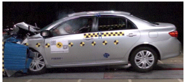
Offset crash test at 64km/h
