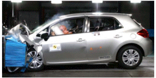
Offset crash test at 64km/h
